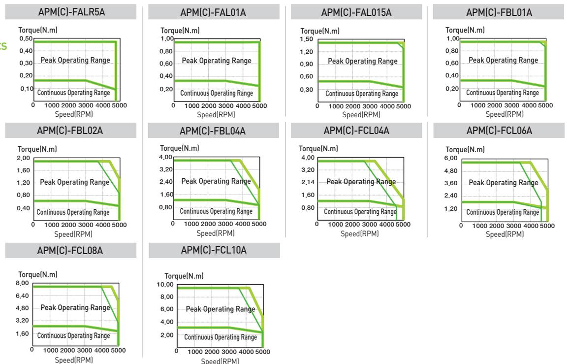
Motor Specifications with Magnetic Absolute Serial Encoder [Rated 2000r/min]
