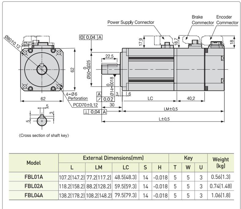
Note1) Use DC[24V] for brake input power supply. Note2) The ( ) is for brake-attached type. Note3) For external dimensions for oil-sealed type. Please kindly contact us separately.
