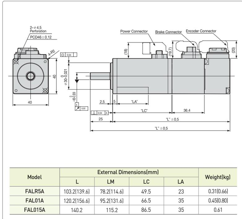
Note1) Use DC[24V] for brake input power supply. Note2) The ( ) is for brake-attached type. Note3) For external dimensions for oil-sealed type. Please kindly contact us separately.
