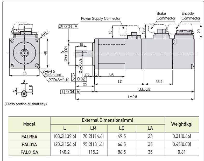
Note1) Use DC[24V] for brake input power supply. Note2) The ( ) is for brake-attached type. Note3) For external dimensions for oil-sealed type. Please kindly contact us separately.
