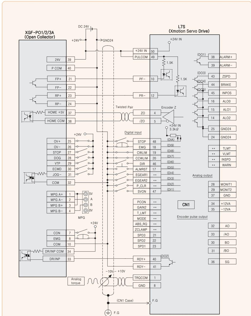
Note1) Input signals DI1 to DIA and output signals DO1 to DO5 are default signals allocated by the factory.
