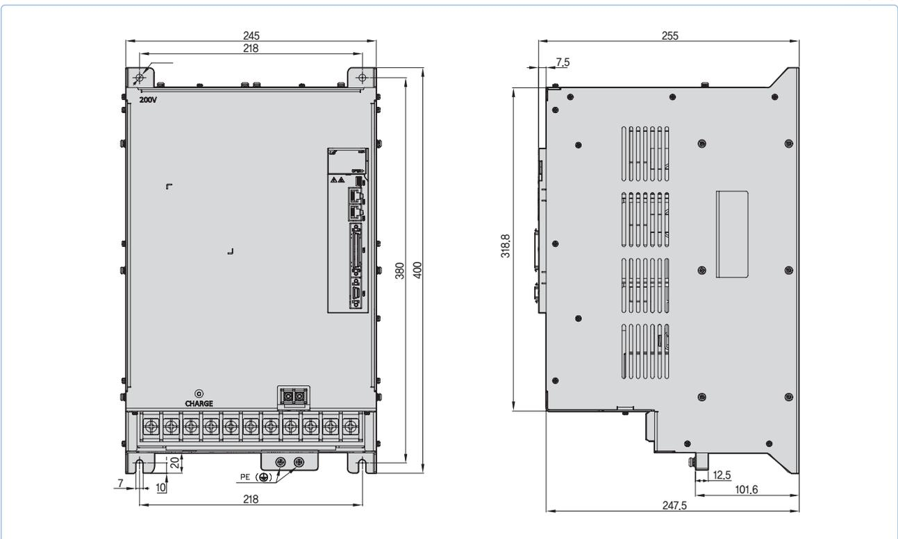
L7SB010B [Weight : 1.5kg(Fan-Cooling included)]
