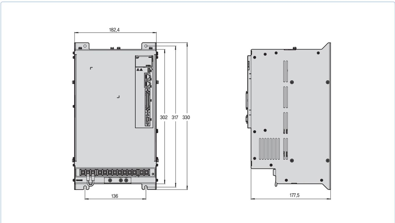
L7SB150B [Weight : 15.5kg(Fan-Cooling included)]
