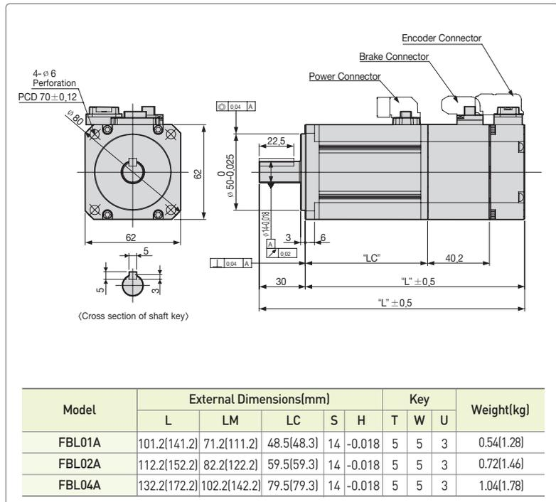
Note1) Use DC[24V] for brake input power supply. Note2) The ( ) is for brake-attached type.
