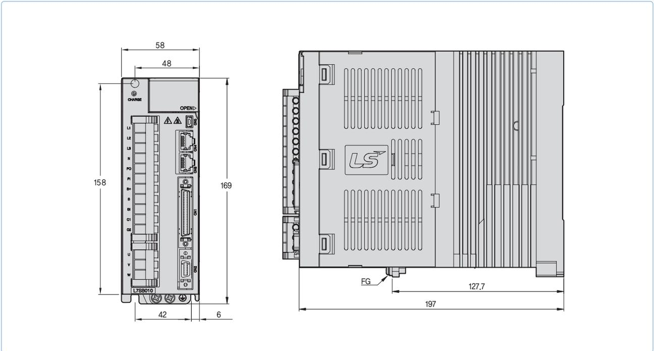
L7SB020B / L7SB035B [Weight : 2.5kg(Fan-Cooling included)]
